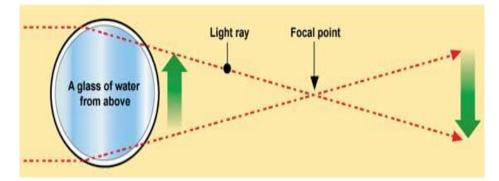
You must think of the glass of water as a magnifying glass. When light goes through a magnifying glass all of the light bends toward the centre. Where the light all comes together is called the focal point. Beyond the focal point, the image appears to reverse. This is because the light rays that were bent, pass each other. The light that was on the right side is now on the left and the left on the right, which makes the arrow appear to be reversed.
